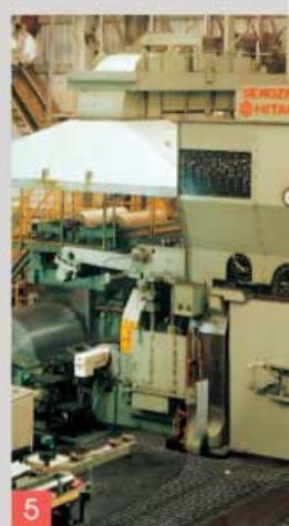
1. | 冷熱軋綜合退火酸洗線 | Cold/Hot Roll Annealing Pickling Line |
